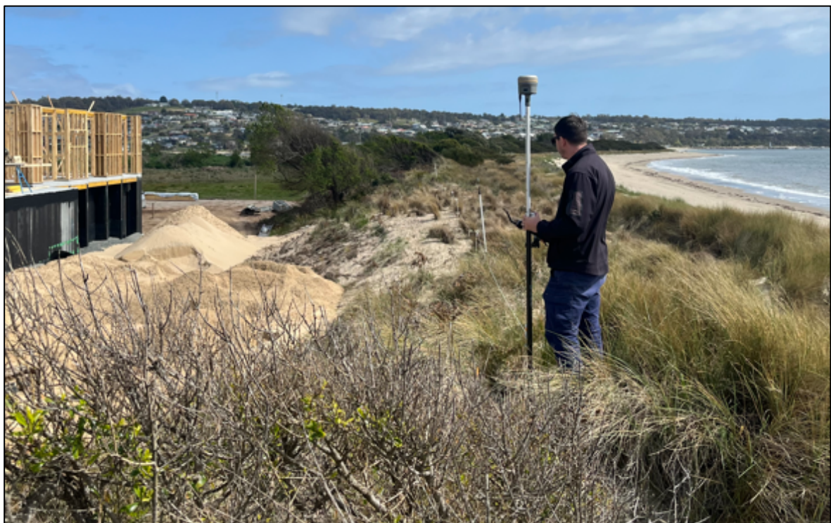
Photo 1 - photo illustrating the location of the survey point taken to reconfirm the location of the northern title boundary at the eastern end of Unit 08.
